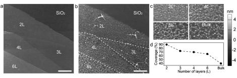
Figure 1. AFM images of BN nanosheets before (a) and after (b) R6G adsorption; c) normalized AFM images with the surface of BN of different thicknesses (number of layers (L)) adjusted to the same height to reveal the different coverage of adsorbed R6G molecules under the same adsorption conditions; d) estimated percentages of coverage versus BN thickness. Scale bars 2 μm.
