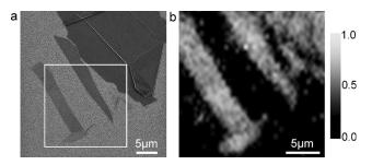
Figure 3. a) Scanning electron microscopy (SEM) image of Ag particles covered by BN of different thicknesses; b) the corresponding Raman mapping from the squared area in (a) after immersion in 10<sup>-6</sup> M R6G solution for 1 h, where 0.0 indicates no intensity and 1.0 indicates the strongest measured Raman peak at 612 cm<sup>-1</sup>.
